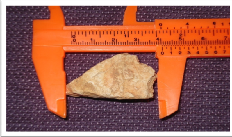
Figure 3.3. Measuring an object using a Vernier caliper.
